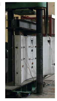
Test of a panelling segment of the extension of Metro Line A in Prague
